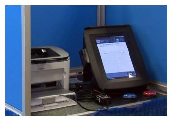
The ImageCast X pictured here with joystick and paddle button accessible voting devices.
