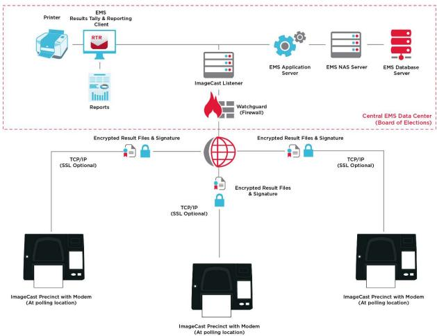
The ImageCast Listener module is responsible for receiving and tracking encrypted results file transmissions from any ImageCast Election Day tabulator.
