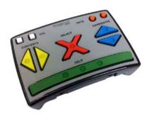
The Audio Tactile Interface (ATI) is the handheld device that is used by a voter during an Accessible Voting Session to navigate through and make selections to their ballot. The ATI:
