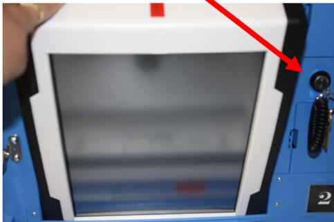
Power the Verity machine on
